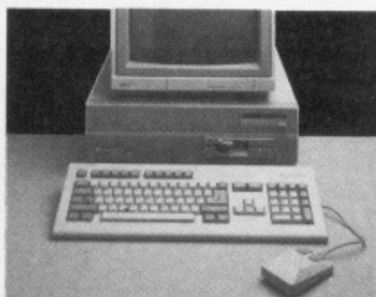
■ Commodore's A2000. Trapped within are specialist chips Fat Agnus, Denise, and Paula
