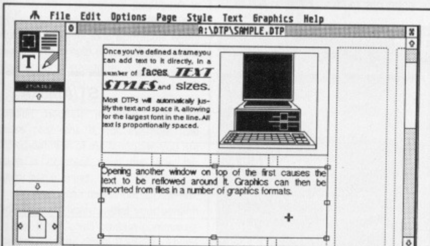
■ Laying another frame over the first automatically re-flows text in the outer frame.
